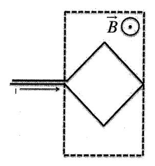
Calculate the force if the metal square has been inserted further into the magnetic field. Everything else remains the same. The square has sides of 1 m, the magnetic field is 0.1 T, and the current is 1 A. Magnetic field is only present in the dotted square as indicated in the figure.
